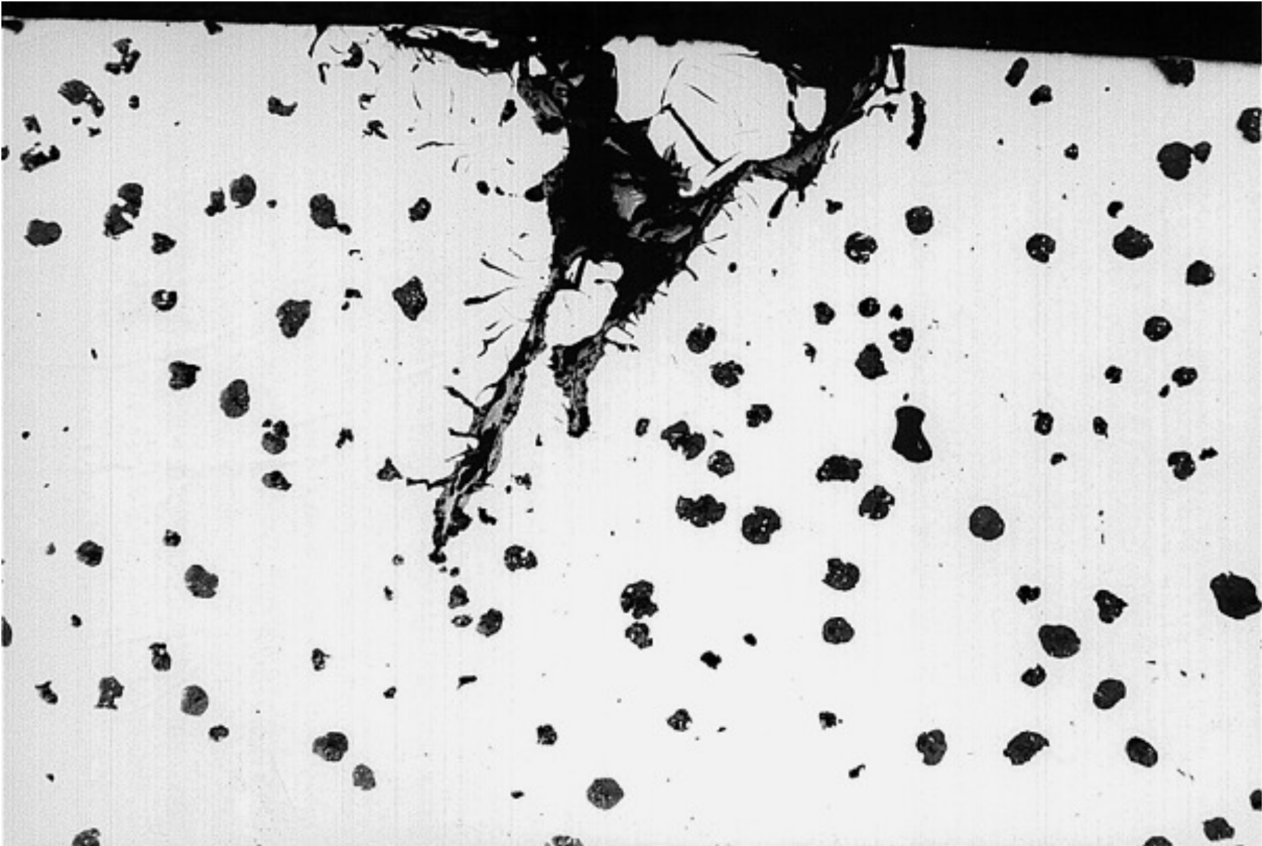
Oxide inclusions in iron
